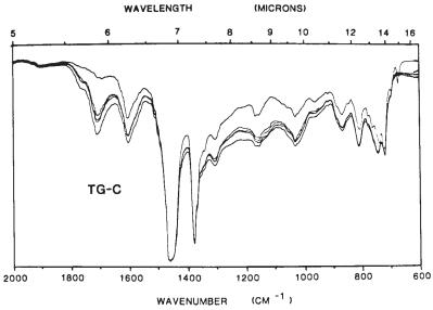
FIG. 5 Crude Oil Progressive Weathering Effects, 0 to 4 Days
